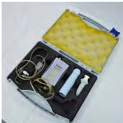
Fig. 1. Picture of the device for anorectal manometry Peritron (Cardio Design Pty Ltd, Oakleigh, Victoria, Australia)
