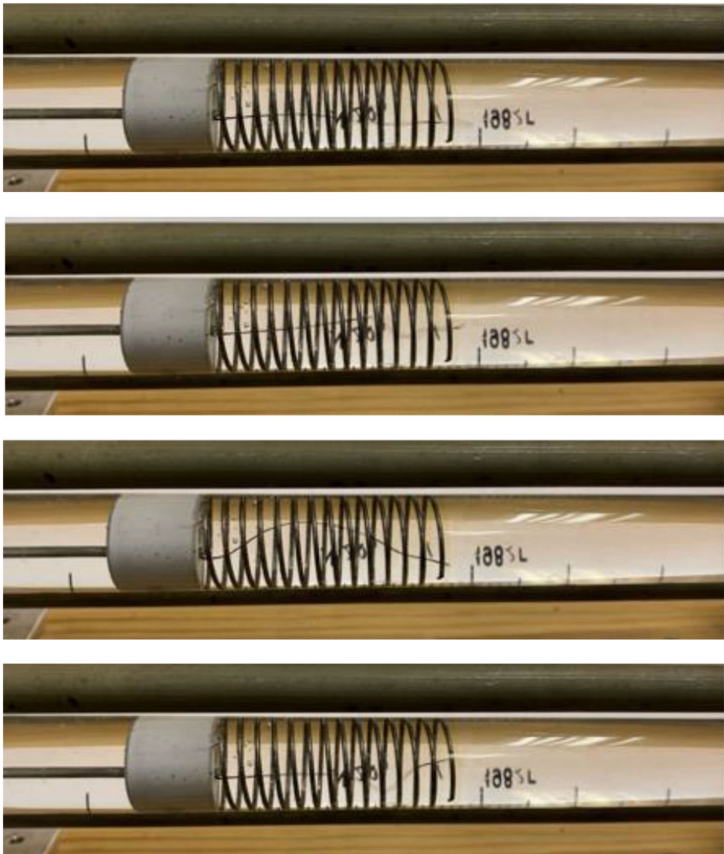
Figure 2. Intravascular stent modeling (endoprosthesis, diaphragm and silk thread are installed inside the rotameter tube). Reflected, standing waves in atrial fibrillation imitation after the pauses for 1,5 seconds and more – the indicator – thread – in different periods of time.
