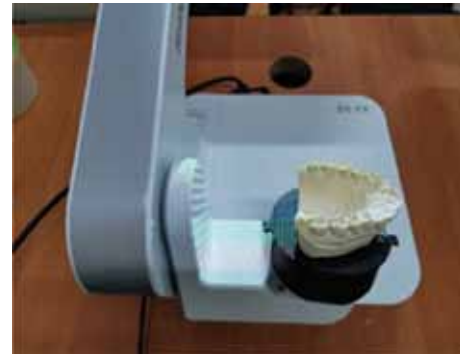
Fig. 8. 3D scanning of a jaw stone model using a Shining 3D scanner
