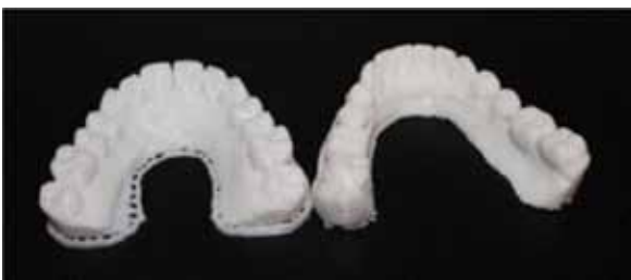
Fig. 11. Printed models of the upper and lower jaws, made using the newly developed technology
